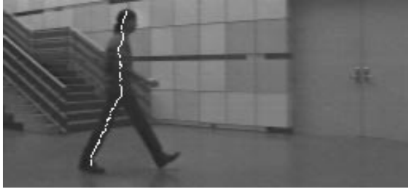
Figure 15: The skeleton model is refined using snakes, with second order discontinuities inserted at the hip, knee, and ankle. The refined skeleton for a particular time instant is shown in white.
