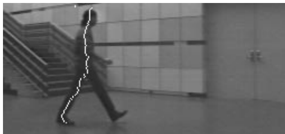
Figure 14: The four body contours are averaged into two skeletons, shown overlaid in white.
