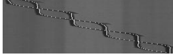
Figure 10: Using the template match as an initial position for the snake, snakes refine the estimate. This yields the centers of both ankles as they move over time. Resulting snakes are shown in white.
