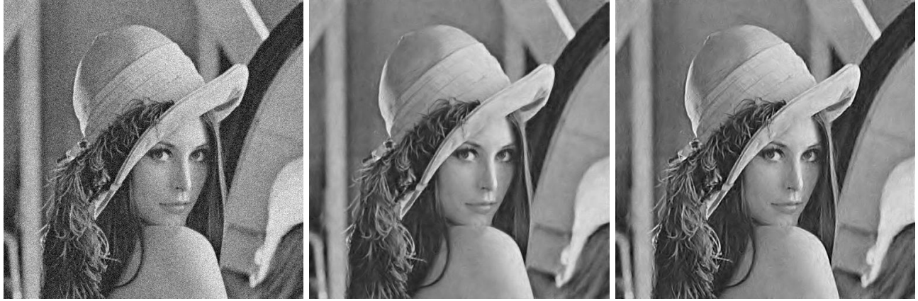
Figure 7. Denoising results. (a) Noisy image, with Gaussian additive noise of standard deviation 20. Noisy PSNR is 22.11dB. (b) Denoised image, using local constraints only. PSNR = 32.47dB. (c) Denoised image, using both local and global constraints. It looks pleasantly sharper, but the PSNR is lower than (b), being 31.13dB.
