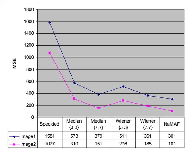
Figure 5. MSE comparison for different filters.
